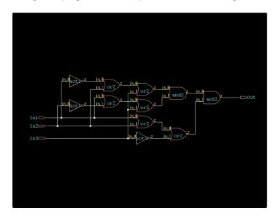
At this point, RTL Compiler has generated an unoptimized version of the Verilog you provided. The final step is "synthesizing" the elaborated design, which optimizes the schematic already created and integrates your design with the AMI standard cell library. While there are many optimization options available to you, we will skip them for this tutorial. The design can be synthesized with the following command:
