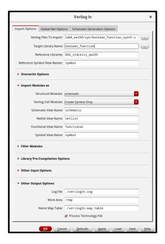
The import process should complete and may have a few errors or warnings. Ignore for now. Go to the schematic cell view created by the import process and open in Virtuoso. The synthesized optimized design should appear with the lowest level of hierarchy being the standard digital blocks (gates) made of transistors in the AMI06 process. If not, something is wrong. **Retry the import process or possibly synthesis before asking for help from the TAs.**
