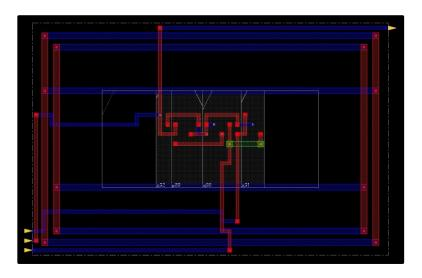
If you see white boxes and spacing errors when you route, your design is too constrained. Consider increasing the offset of your power rings by increments of 0.15.
