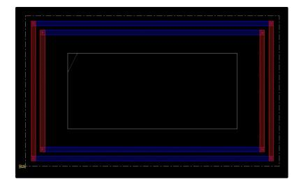
Connection to the global nets is done automatically if the nets are given the same names as was done in the setting of the power nets above. If all was done correctly, power planning should be finished.
